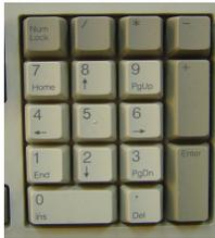
At the far right side of the keyboard is the number keypad. It is a keypad like you would find on a calculator. This is to make it easier to rapidly enter numbers. The five (5) key has a little bump on it so that you can find your “home” position (your middle finger on the five key) without looking (you can feel the bump with your middle finger). This is like the bumps on the “F” and “J” typewriter keys, which are for the same purpose.
