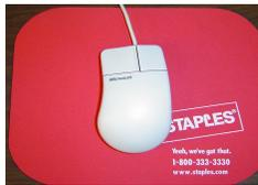
The roller mouse has two rollers inside it, one at the top or bottom and one at the side. A rubber ball rests on these rollers inside the mouse, and touches the mouse pad outside. Moving the mouse moves the ball, which moves the rollers. When the rollers spin, that tells the computer to move the pointer on the screen. A laser mouse simply has a laser shining on the mouse pad or table to notice when the mouse moves.
