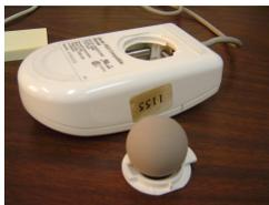
The ball in a roller mouse is rubber with a heavy metal center. It can be removed by loosening the cap on the bottom of the mouse and turning the mouse over. The ball will fall out. If you forget to put your hand under it it will roll across the floor. Clean the ball with soapy water and dry with a towel. You can also clean the rollers with a q-tip or your finger nail. Laser mice do not have a ball.
