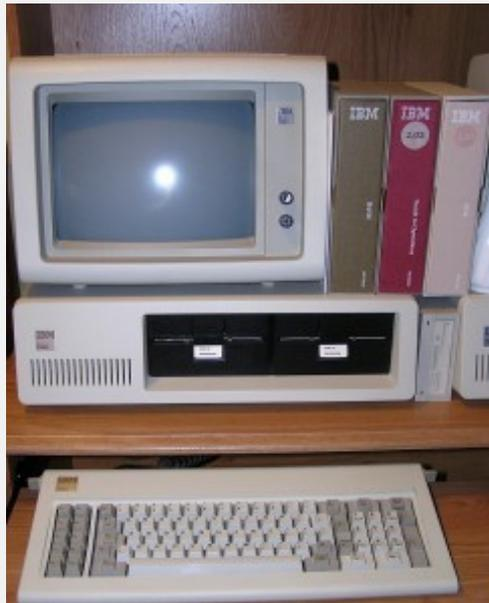
IBM 5150 Personal Computer System With IBM 5151 Monochrome Display Keyboard DOS 2.1 Guide To Operations And Basic Manuals. Public Domain.
