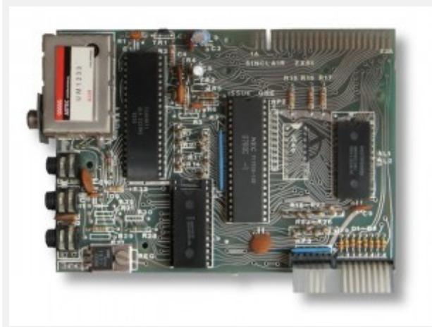
Manually designed ZX81 printed circuit board. A later version was made using CAD tools. Public Domain.
