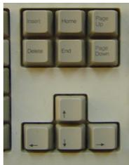
To the right of the main keyboard is a set of keys used to move around in spreadsheets and word processing programs. There are four arrow keys at the bottom and six keys together at the top marked **PGUP** (Page Up), **PGDN** (Page Down), **HOME** (go to the beginning), and **END** (go to the end).
